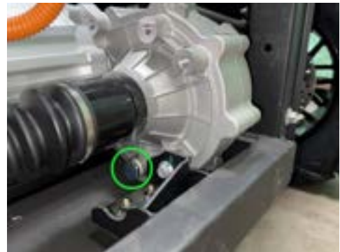
Front gearbox oil drain plug location (Shown with front bumper removed)
