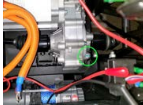
Front gearbox oil fill plug location (Shown from above with hood removed)
